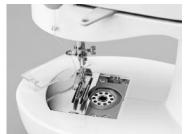
The machine may have come pre-threaded from the factory. Look at this threading carefully before removing it to replace the thread or bobbin with different thread. Then follow the preceding instructions to rethread.
